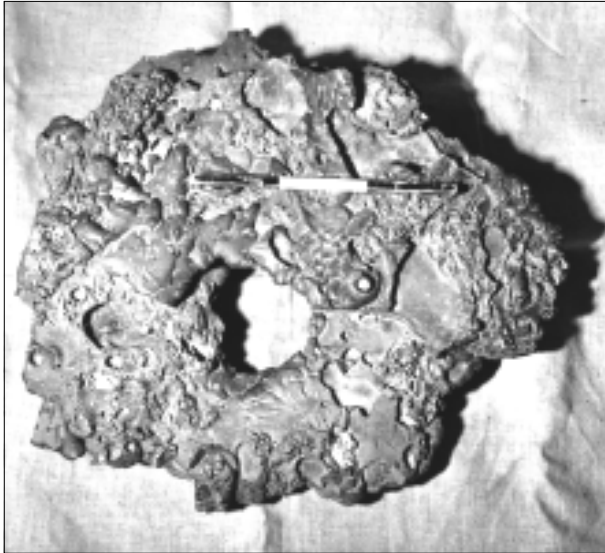
Fig. 24. Slag 'cake' with cast-in centre hole. Site 2.
