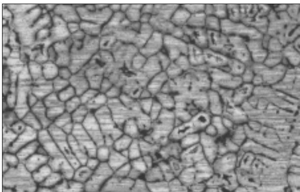
Fig. 7. Equi-axed grain structure of ingots showing that they were cast in the mould, metallographic microscope, x125.
