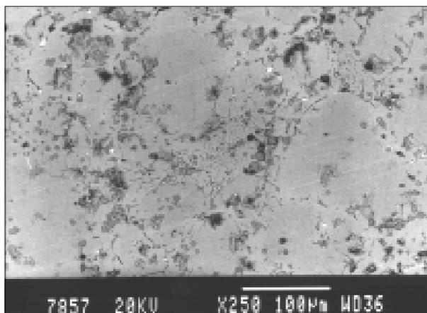
Fig. 12. Surface of Ingot 6 showing Cu<sub>2</sub>O-Cu eutectic structure (BEI).
