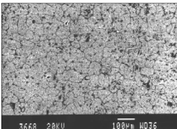
Fig. 5. Structure of the middle part of Ingot 13 with wide triangular section showing absence of lead inside of it (BEI).
