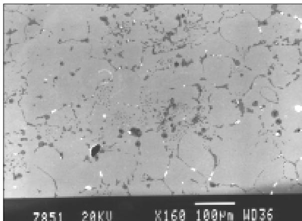
Fig. 10. Etched surface of ingots 2 and 5 revealing presence of black iron oxide inclusions within copper sulphide. Rare white droplets are lead (BEI).
