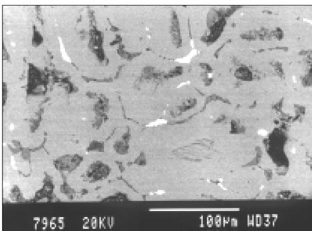
Fig. 8. Same as fig. 7 showing presence of copper sulphide (gray) and lead (white) inclusions in the grain boundaries (BEI).
