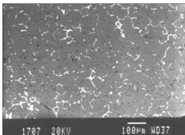
Fig. 6. Structure of ingots with thin elongated form of section. Lead is distributed throughout the ingot (BEI).
