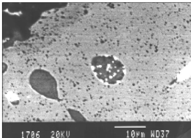
Fig. 9. Complicated structure of copper sulphide inclusions with numerous small lead spherules inside (BEI).
