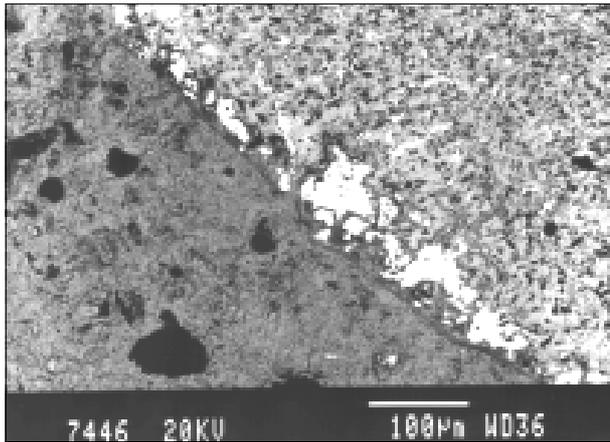
Fig. 3. Typical upper crust structure: external gray layer is copper oxide, white – lead and internal light gray layer is copper. Dark gray and black inclusions are remnants of the slag (BEI).
