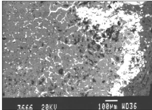
Fig. 4. Penetration of lead (white) through the copper grains from middle part of the ingot to the surface (Ingot 13, for example, BEI).
